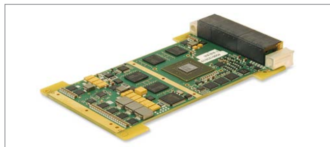
Figure 1 | The Abaco Systems GRA113 3U VPX rugged high-performance graphics board features a 640-core GPU from NVIDIA.
