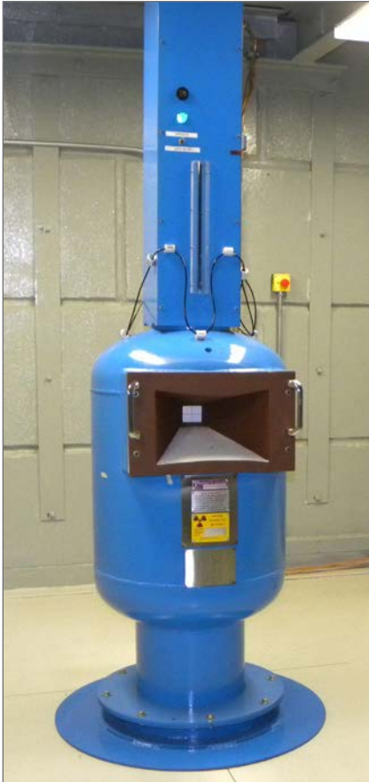
Figure 2 | Low-dose-rate radiation testing of components enables designers to screen parts for suitability for use in space. Photo courtesy of VPT Rad.
