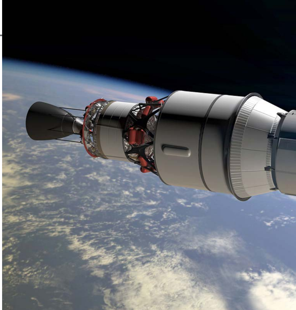
The Orion Crew Module EFT-1 test vehicle stack contains the crew module, the service module, a partial launch-abort system containing only the jettison motor, and the Orion-to-stage adapter. (Photo credit: NASA.)
